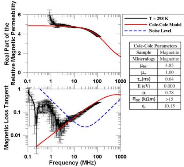
Figure 2. Temperature independent magnetic relaxation losses in magnetite (density = 2.62 g/cc). The error bars represent the 68.2% confidence intervals or  $\pm 1$  standard deviation. The parameters for the Cole-Cole model are listed below the legend.
